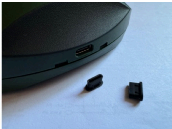
The USB-C rubber plug installed in the PUC
