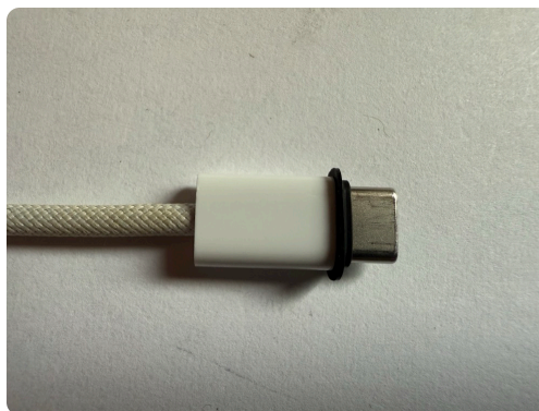
An o-ring sealing a USB-C cable to the PUC
